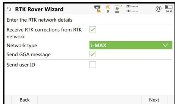
The Network type **i-MAX** = Network RTK Corrections from Multiple Network RTK Base Stations, based on your RTK Rover’s position. The Network RTK Server computes these **i-MAX** RTK Corrections, sends them to the Network RTK Rover.
