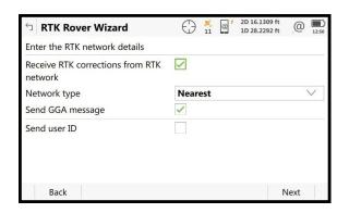
The Network type **Nearest** = Single Baseline RTK Corrections from the Closest Network RTK Base, Based on the RTK Rover's position.
